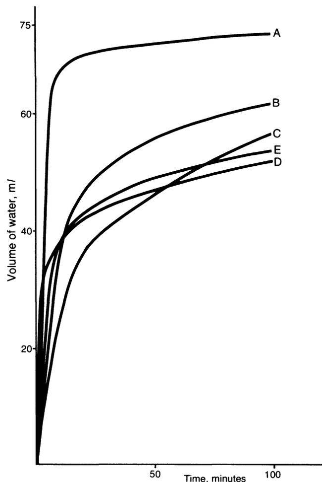
**Figure 5. Emulsion-breaker test—Procedure I.3. AL 150°C 75% water. T = 20°C. Emulsion breakers at 1,000 ppm.**
