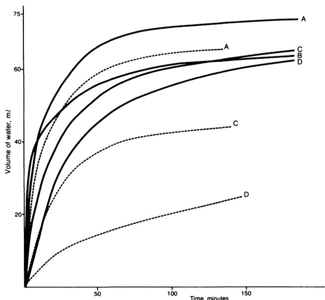
**Figure 4. Emulsion-breaker test—Procedure I.2. AL 150°C 75% water. Solid line, T = 21°C; broken line, T = 12°C. Emulsion breakers at 1,000 ppm.**
