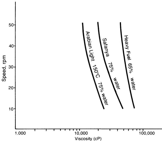
Figure 1. Brookfield viscosity of different emulsions at 20°C.
