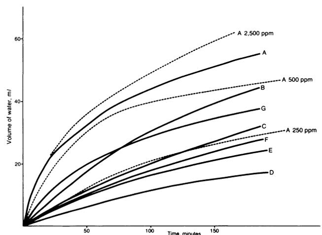
Figure 3. Emulsion-breaker test—Procedure I.1. AL 150°C 75% water. T=21°C. Emulsion breakers at 1,000 ppm except as indicated.
