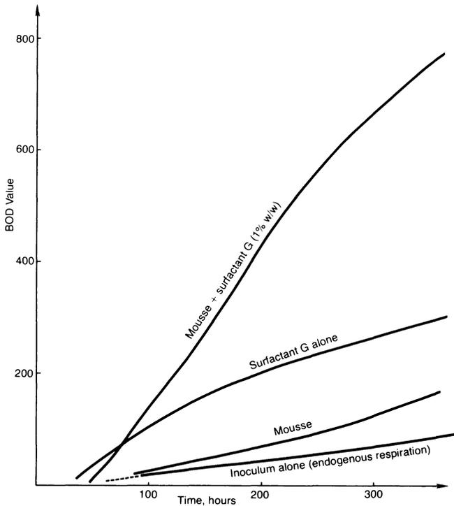
**Figure 9.** Oxygen consumption measured under agitation in artificial sea water supplemented by nutrients and inoculated.
