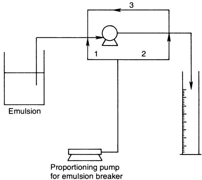
Figure 2. Schematic of laboratory test of emulsion breakers.
